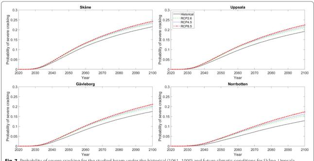
Fig. 7 Probability of severe cracking for the studied beam under the historical (1961–1990) and future climatic conditions for Skåne, Uppsala, Gäyleborg, and Norrbotten
