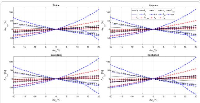
**Fig. 12** Percentage change in the mean value of the end-of-century corrosion rate due to changes in the mean value of the different input parameters in the corrosion initiation and corrosion rate models considering the historical climate (1961–1990)
