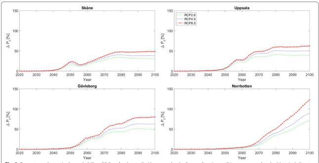
Fig. 9 Percentage change in the probability of failure for the studied beam under the future climatic conditions compared to the historical climate (1961–1990)
