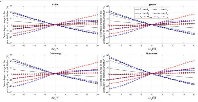
**Fig. 10** Percentage change in the end-of-century probability of corrosion initiation due to changes in the mean value of the different input parameters in the corrosion initiation model considering the historical climate (1961–1990)
