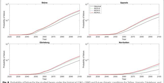
Fig. 8 Probability of failure for the studied beam under the historical (1961–1990) and future climatic conditions for Skåne, Uppsala, Gävleborg, and Norrbotten
