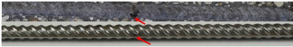
Fig. 9 Before and after cleaning rebar in specimen FA-8 [18, 23]
