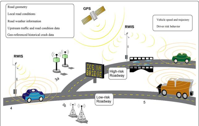
**Fig. 1** Conceptual design of next-generation highways in cold climates. Application scenarios include safety applications (e.g., blind spot warning and collision warning) and mobility applications (e.g., traveler information, routing support, and coordinated truck platooning [not shown])
